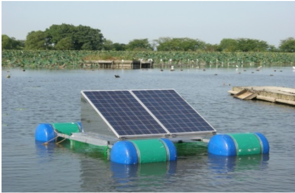
Fig. 1: Operation of equipment by solar energy (Lake Hyoko, Niigata Prefecture)
